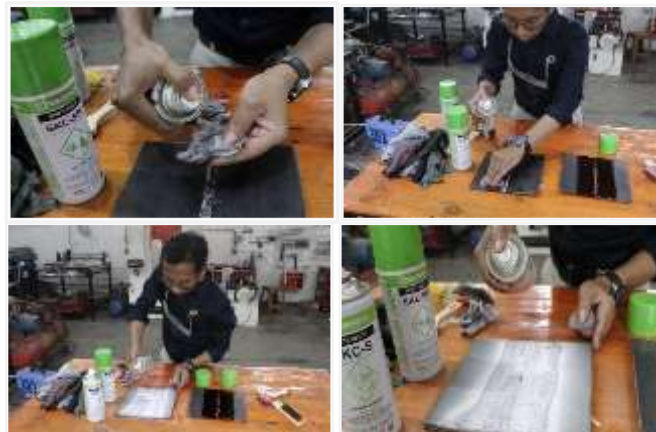
Gambar 1. Pengujian NDT ( Non Destructive Test-Penetrant Test )
